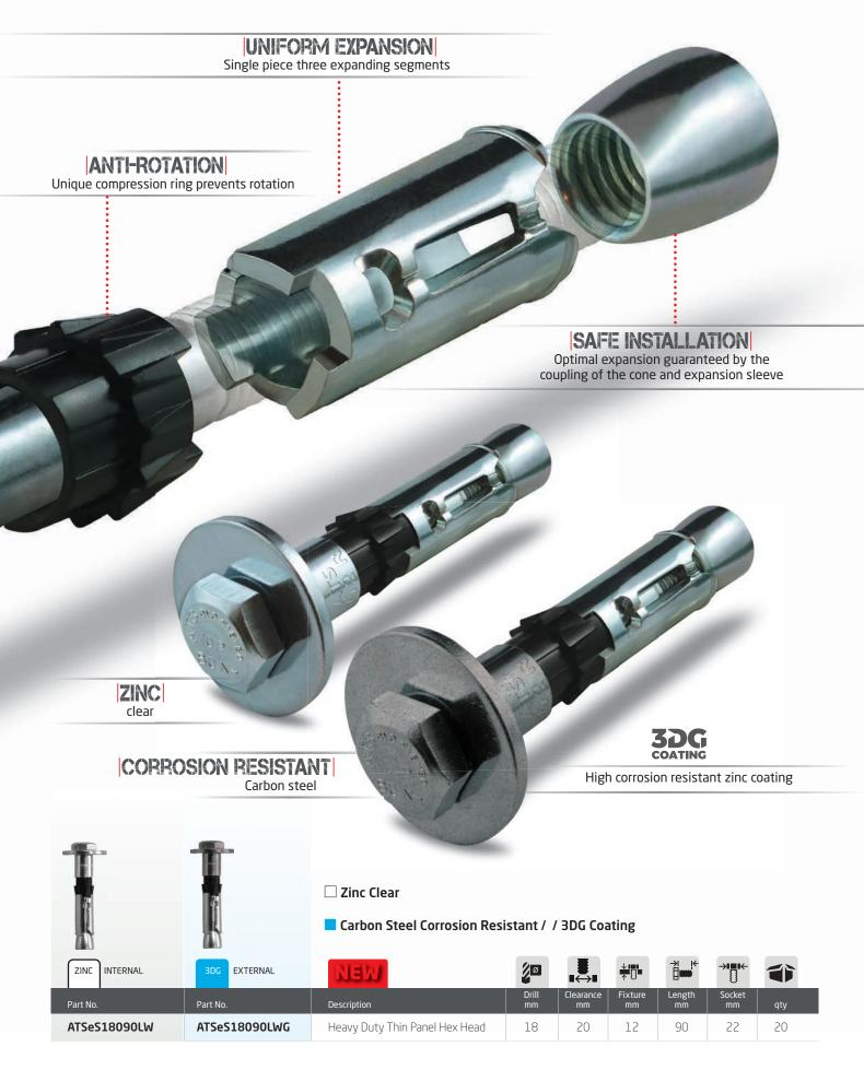
HEAVY DUTY SAFETY ANCHOR FOR THIN PRECAST CONCRETE PANELS
